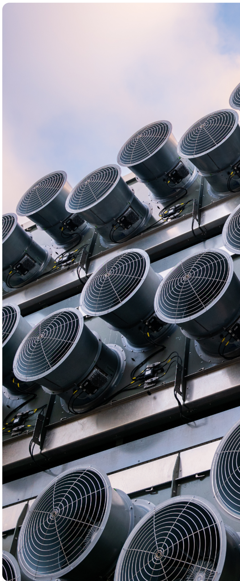
Direct air capture (DAC) is the use of chemical or physical processes to extract carbon dioxide directly from the ambient air. The extracted CO 2 is then sequestered in safe long-term storage.
