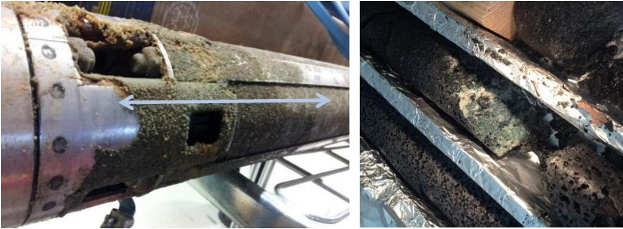
*Figure 11: Precipitates collected from a submersible pump in a Monitoring Well during the original Carbfix pilot injection after it was hauled to the surface. X-ray diffraction and scanning electron microscopy confirmed these precipitates to be calcite with similar  $^{14}\text{C}$  concentration of the injected  $\text{CO}_2$  and the precipitated collected calcite.*
