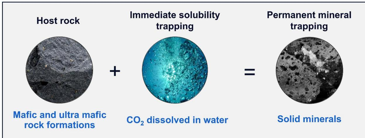
Figure 8: Simplified diagram of in-situ carbon mineralization (Carbfix)
