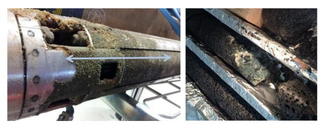
Figure 11: Precipitates collected from a submersible pump in a Monitoring Well during the original Carbfix pilot injection after it was hauled to the surface. X-ray diffraction and scanning electron microscopy confirmed these precipitates to be calcite with similar <sup>14</sup>C concentration of the injected  $CO_2$  and the precipitated collected calcite.
